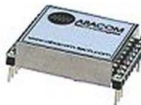
Pin Spacing: 2.54mm (0.1") Pin diameter: 05mm
